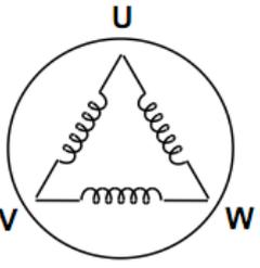
A schematic diagram of a three-phase motor winding in a delta configuration. It consists of a circle containing an equilateral triangle. Each side of the triangle is represented by a wavy line, indicating a winding. The vertices of the triangle are labeled with the letters U, V, and W. U is at the top vertex, V is at the bottom-left vertex, and W is at the bottom-right vertex. |
