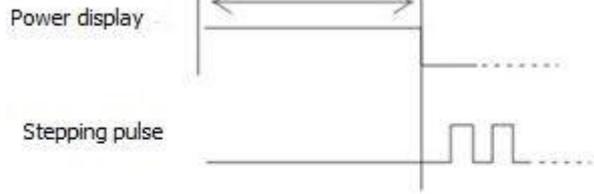
Note: Driver power-up time depends on the applied AC driver voltage magnitude, under 36V power-up time need 2 seconds typically.
