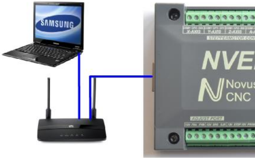
Figure 2-14. Connect in Router mode
