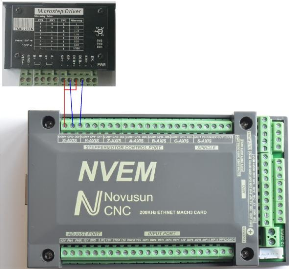
Figure 2-3. Stepper driver connection
