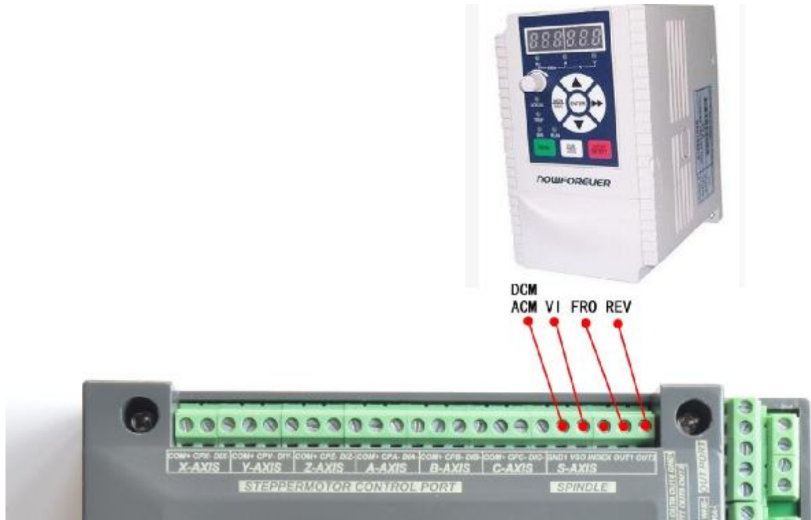
Figure 2-4. spindle control output and inverter connection
