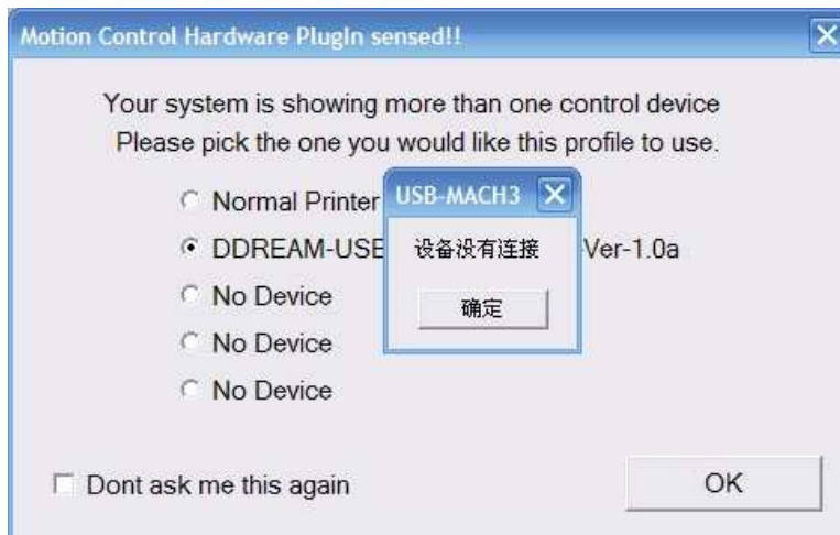
Figure4-2. Not connected correctly
