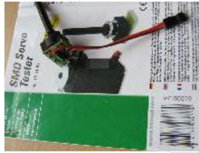
This is a tsunami 25 amps esc . Normally driven with a RC receiver. Now driven by the Conrad Servo tester
