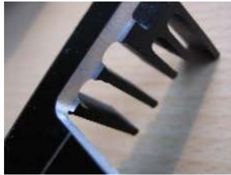
CNC - cut of course..... .....on my Bracket machine using a 5mm single side cutter
