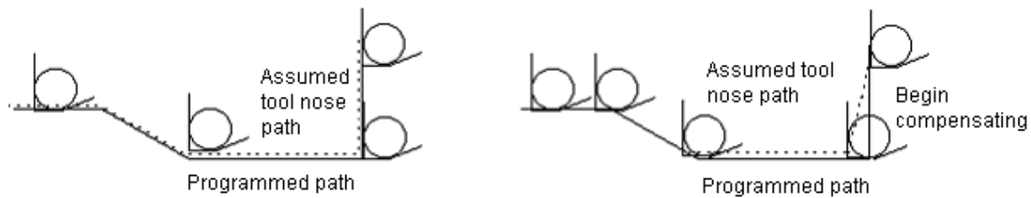
Fig. 4-6-1-1-4 Tool path during the imaginary tool nose programming
