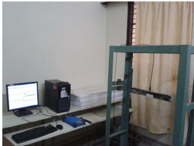
Fig.4. Experimental setup for vibration analysis
