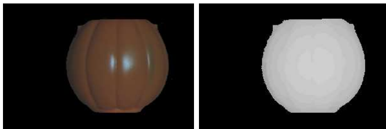
Figure 17: The ground truth dataset. Left is one color image and right is its corresponding depth map. Bad pixels due to occlusions are manually removed.
