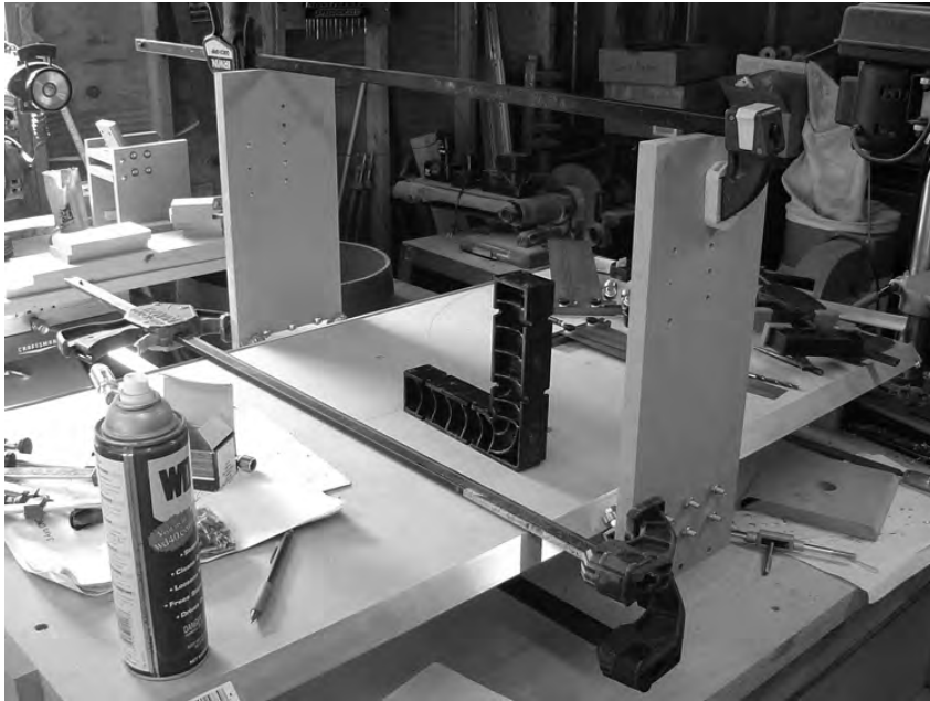
Figure 11-5. Mount the gantry sides (Parts Q and R) to the table.
