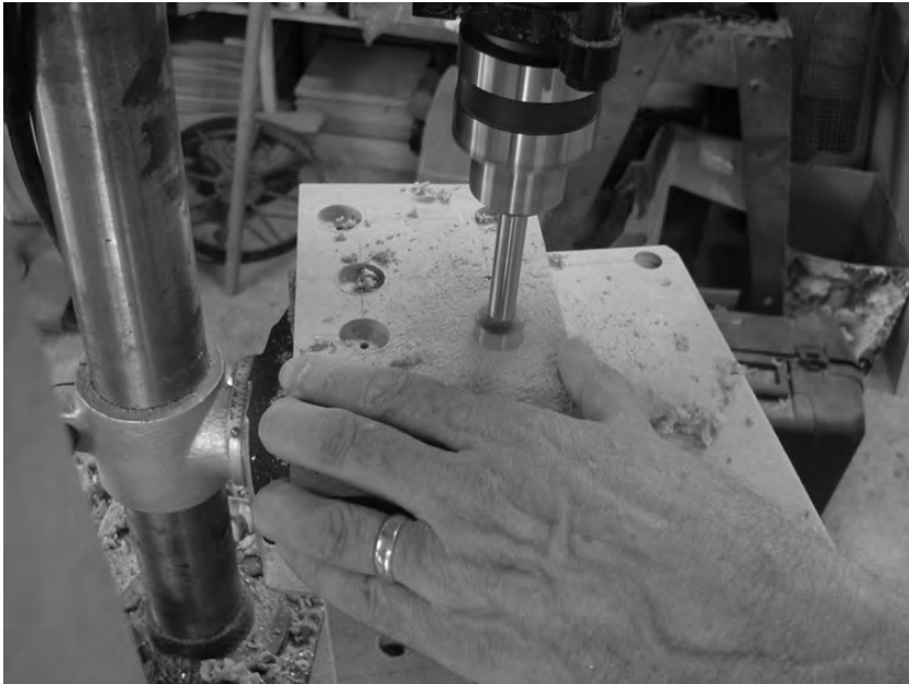
Figure 13-6. Drilling the counterbored holes in Part C
