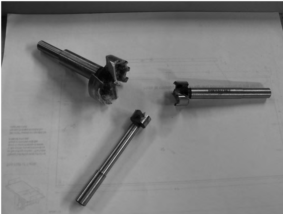
Figure 2-1. Forstner drill bits in various sizes
