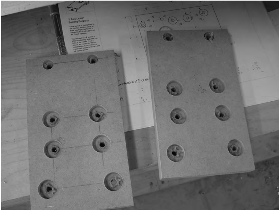
Figure 13-8. Counterbored holes with 1/4" drilled centers
