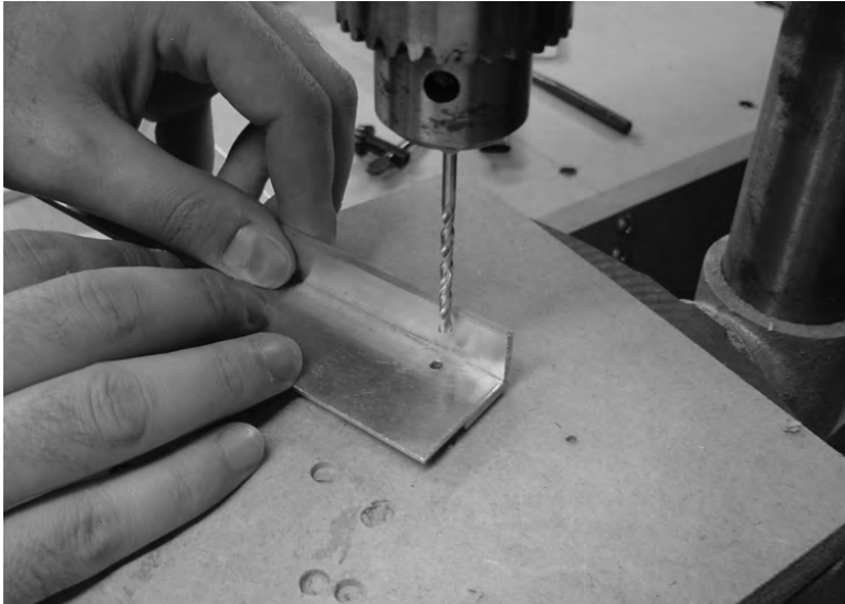
Figure 10-10. Drilling pilot holes into the BRA rails
