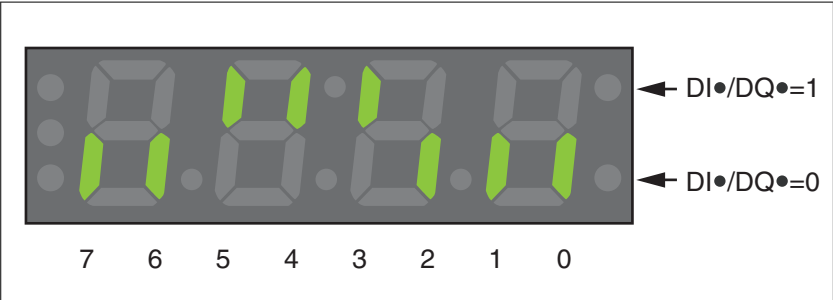
Figure 43: Integrated HMI, displaying the signal state of the digital inputs (DI•) and outputs (DQ•)
