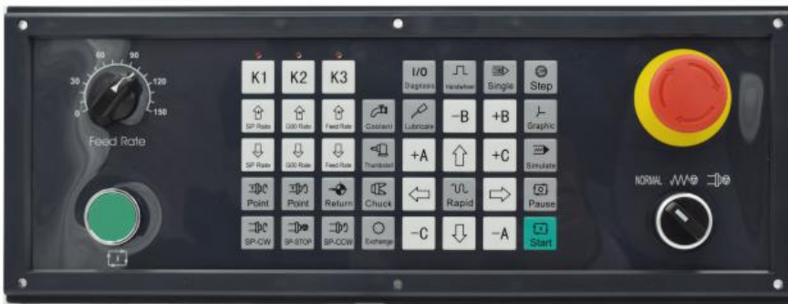
C Type Operational Panel
