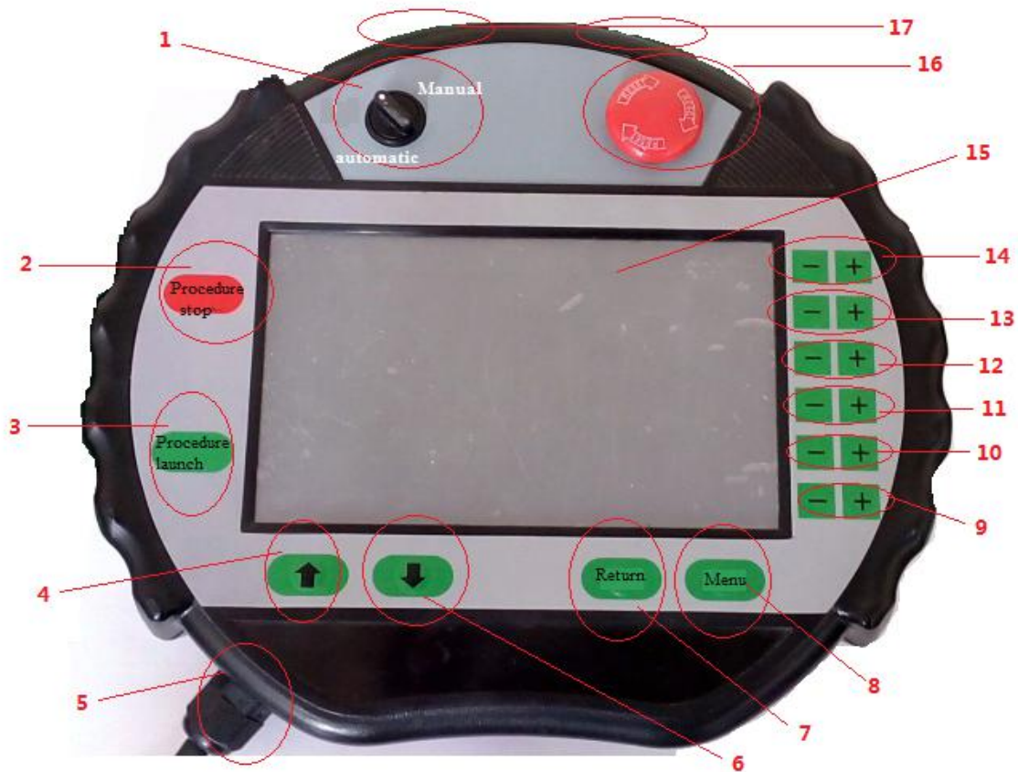
Fig. 2.2 Composition Structure of Demonstration Box
