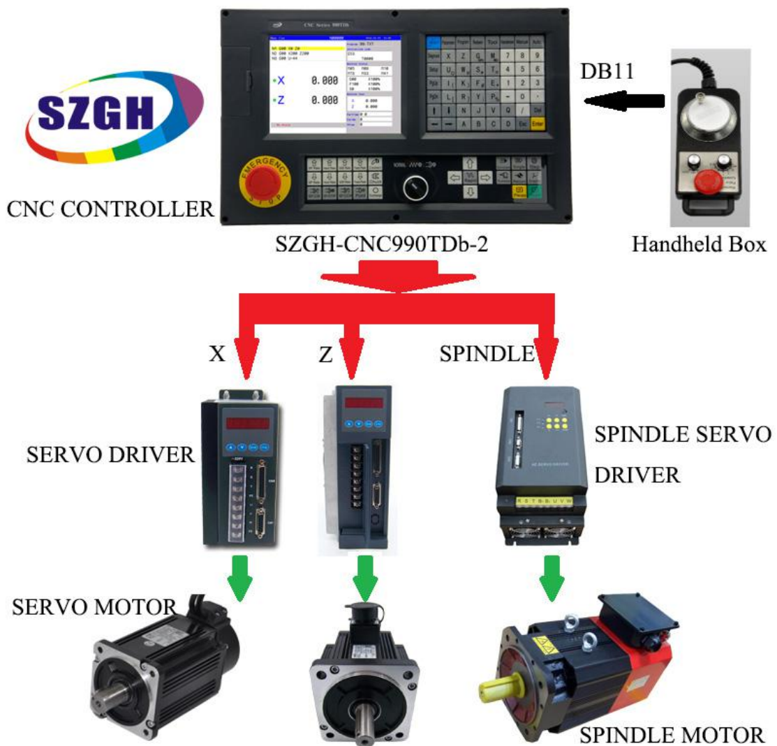
Fig1.2 Wiring Sketch for Total CNC Lathe System
