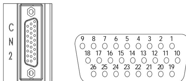
Figure 3-2 The view and layout of the CN2 I/O interface terminal
