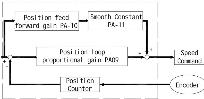
Figure 5-6 Flowchart of the position control loop
