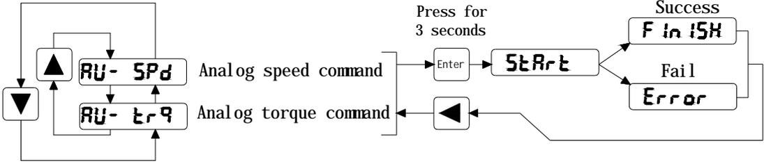
Figure 4.8 Diagram for the operational processes of analog zero-offset adjustment
