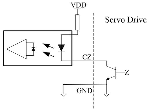
Figure 3-11 Encoder Open-collector Z-pulse output interface circuit type 6
