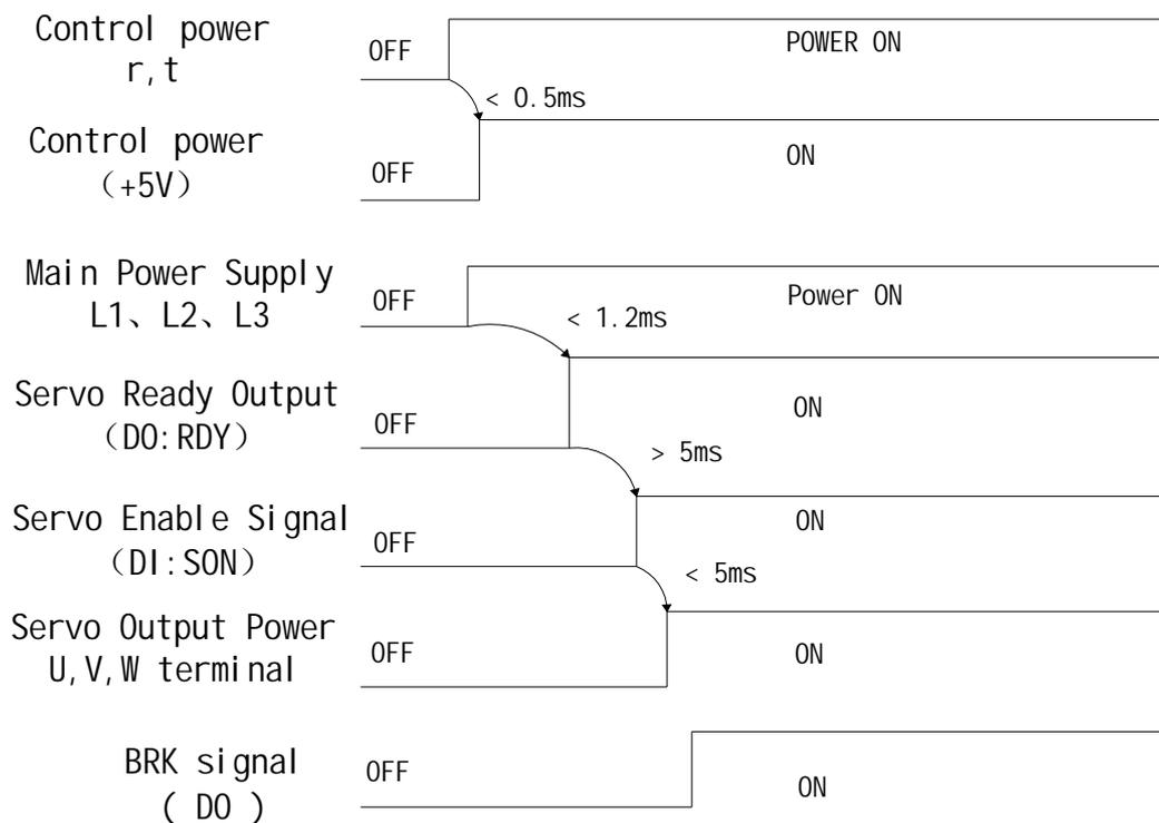
Figure 5-10 Timing flowchart about drive power on
