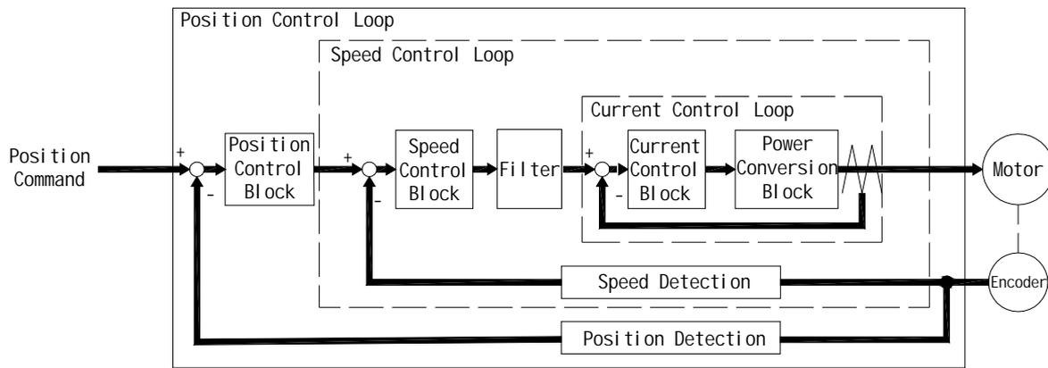
Figure 5-7 Diagram for the servo closed-loop control system
