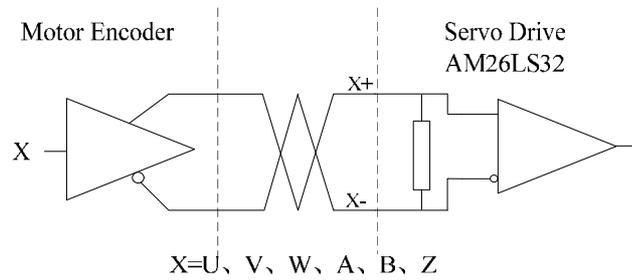
Figure 3-12 Encoder feedback signal input interface circuit type 7
