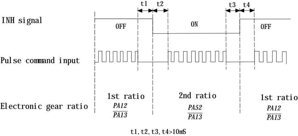
Figure 5-5 Diagram for dynamic electronic gear ratio
