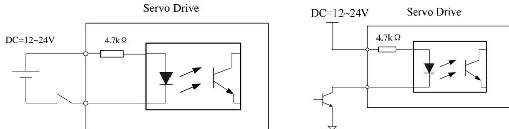
Figure 3-3 Digital signal input interface circuit type 1
