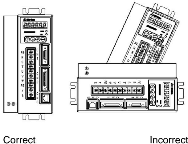
Figure 2-3 The correct direction for installation Minimum Clearances
