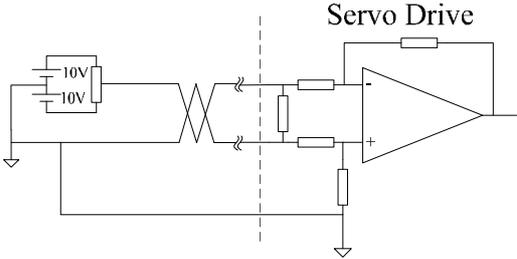
Figure 3-7 Analog signal input interface circuit type 4 ( differential input mode )
