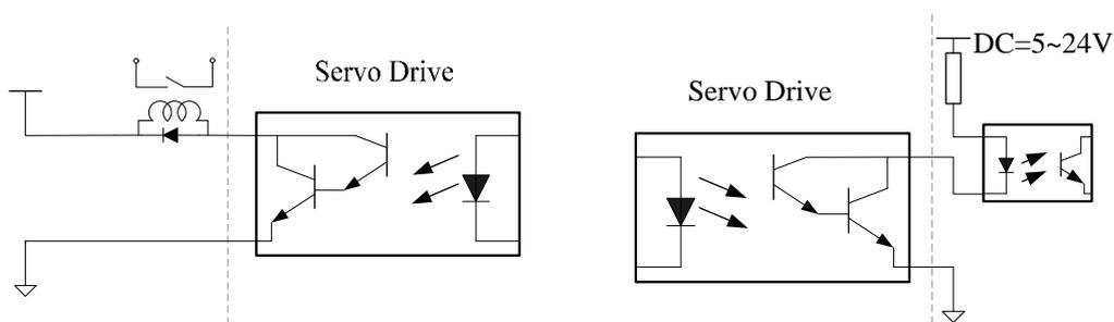
Figure 3-4 Digital signal output interface circuit type 2
