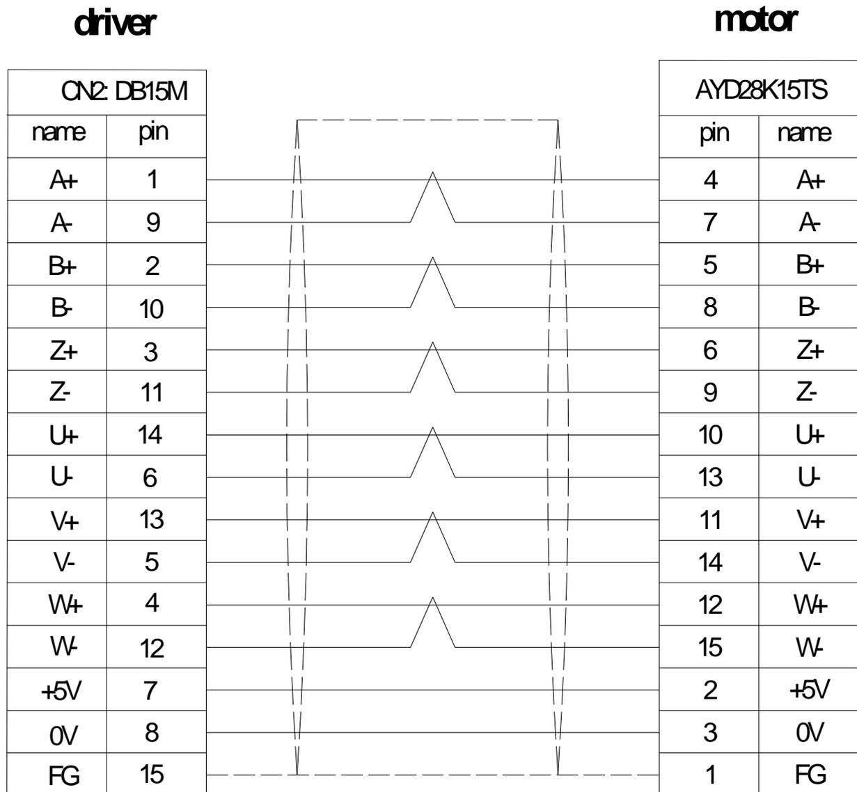
Figure 9-1      Connecting diagram for encoder cable between Hiriden drive and motor
