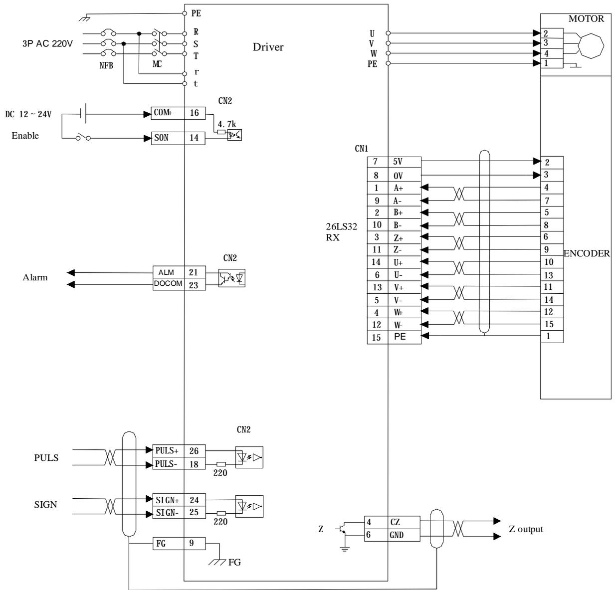
Figure 5-3 wiring diagram for the simple position control system
