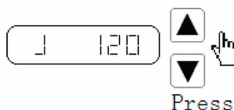
Figure 4.7 Diagram for the JOG trial run
