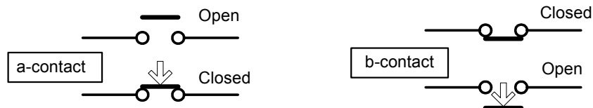
Fig. 9- 7 The operation diagram of a-contact and b-contact
