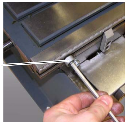
Illustr.6-11: Disassemble limit stop
