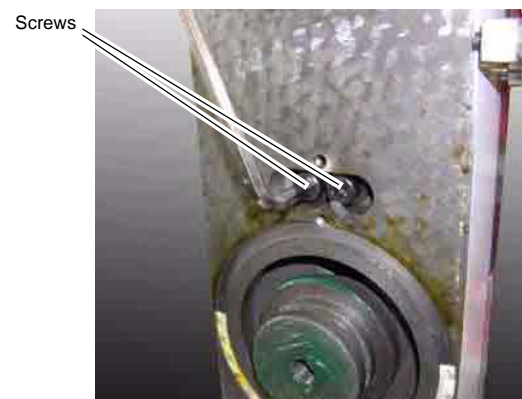
Illustr.6-71: Loosen screws
