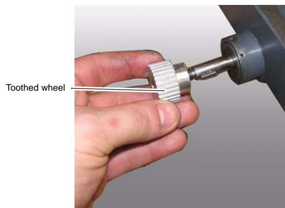
Illustr.6-5: Disassemble toothed wheel
