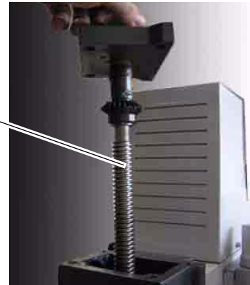
Illustr.6-66: Unscrew spindle
