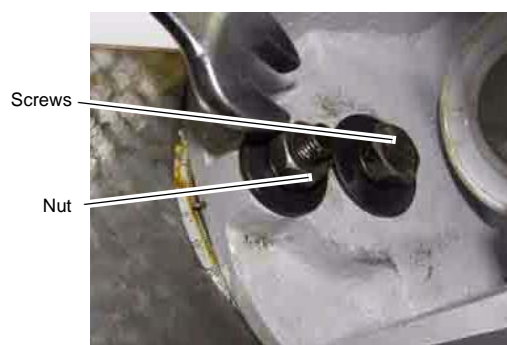
Illustr.6-86: Clamp milling head
