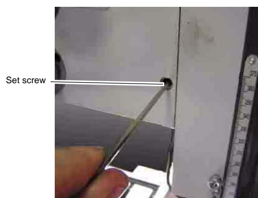
Illustr.6-68: Loosen set screw
