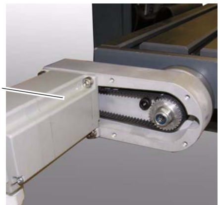
Illustr.6-3: Step motor left hand side
