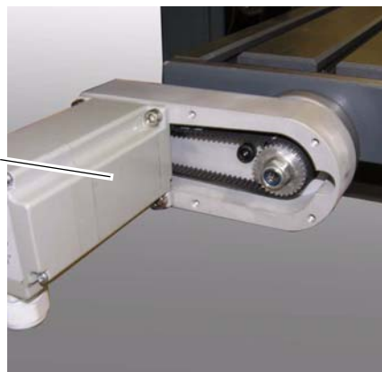
Illustr.6-63: Mount step motor
