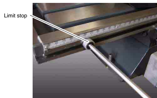
Illustr.6-60: Screw on limit stop
