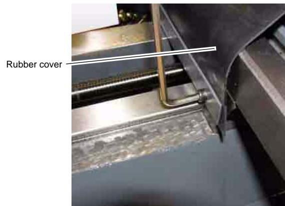
Illustr.6-59: Assemble rubber cover
