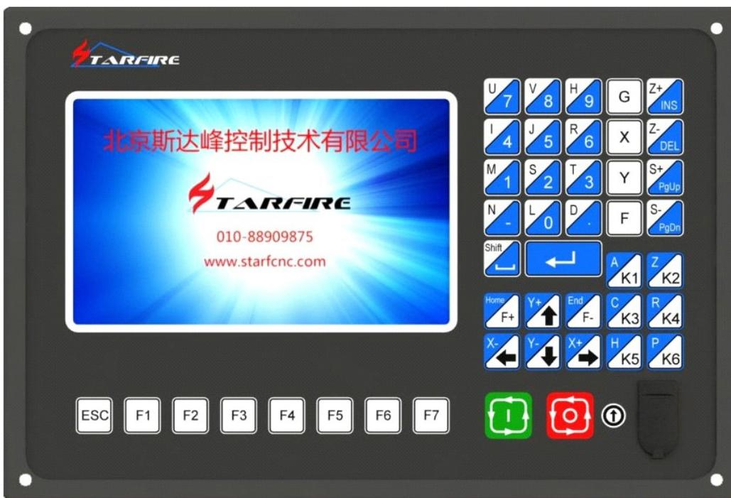
【F1】 - 【F8】 : Function keys, under different interface, with the corresponding prompt functions;
