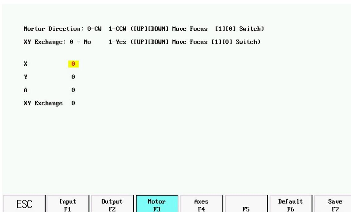
In the figure above, press 【↑】【↓】 to move the cursor, press [1] [0] to change the direction, and press [save] after setting.
