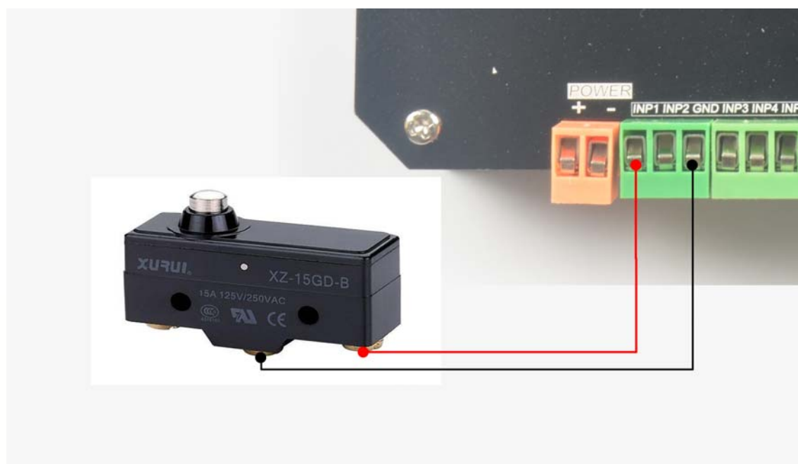
Figure2-4. Probe/Estop/ ordinary fretting switch input connection
